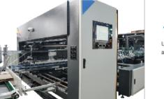
Upper and lower belt can move forward and back motorized as well as the thickness adjustment to adapt to different kinds of box.
