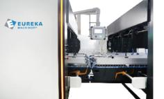
4/6 corner folding system with intelligent servo-motor technology. It allows accurate folding of all back flaps by means of hooks installed in two independent shafts controlled electronically.
