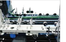
Squeezing unit in the folding unit can minimize the fault created by slotting unit or rotary die-cutter of traditional Flexo printer.
