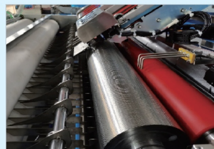
Glue system with extra large 160mm diameter anilox roller with 150mm pressing roller(*EUFM PRO) Glue coating value can be set on touch screen and control precisely by servo motor.
