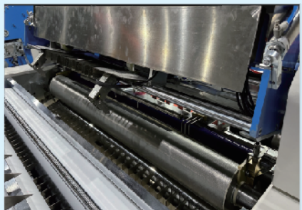
Automatic detection of top and bottom with servo correction technology
