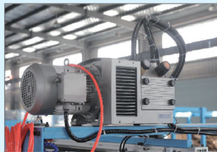
Top Sheet Feeding Mechanism with Becker pump
