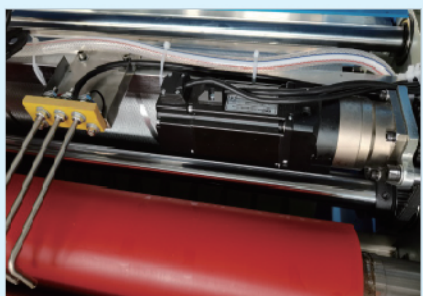
Glue system with extra large 160mm diameter anilox roller with 150mm pressing roller(*EUFM PRO) Glue coating value can be set on touch screen and control precisely by servo motor.
