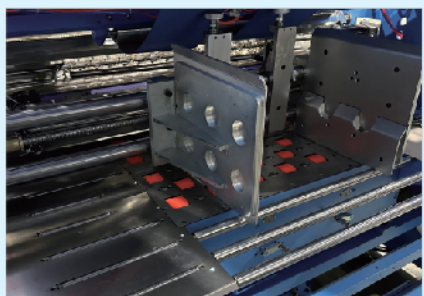
Lead edge feeding system with non-pressure structure
