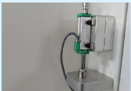
Board thickness auto adjustment with detection
