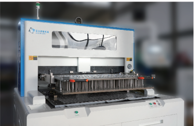
Use 3 or 5 mm stripping pin which fit to different job easily.
